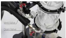
Quick and easy to drain thermal fluid.
