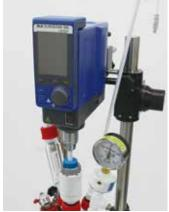
Simply attach an overhead stirrer for motorized mixing.
