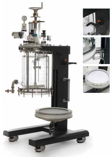
Operator can adjust and align the filter unit without tools. You need not make frequent filter adjustments. The swinging mechanism helps with filter access, and you can retrieve the cake easily.
