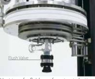
Heat transfer fluid runs from top to bottom. Flush Valve minimizes dead space.
