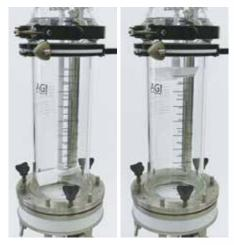
Lower and lift the shaft easily using one hand. This allows for easy simple height adjustment for stirring shaft.
