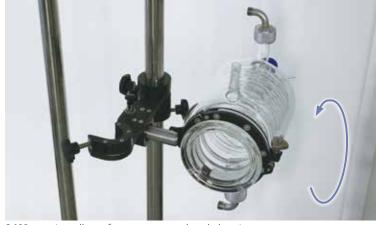
360° rotation allows for easy removal and cleaning.
