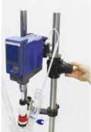
Lower and lift the motor and/or vessel easily using one hand. This allows for easy preparation and cleaning.
