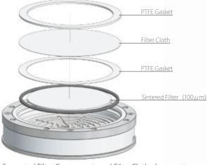
Separated Filter Components and Filter Cloth placement.
