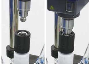
AG! designed Flexible Bearing Coupling creates flexibility between the motor and stir shaft allowing for efficient stirring even is the motor and connection is not aligned perfectly.
